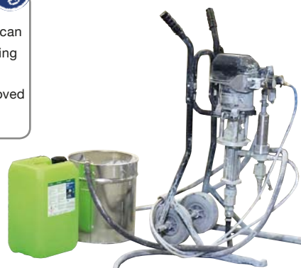
Hose system cleaning with PROLAQ Liquid
